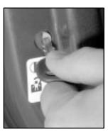
2. Turn the lock counterclockwise with your ignition key to engage the safety lock. Turn the lock clockwise with your ignition key to disengage the safety lock.
